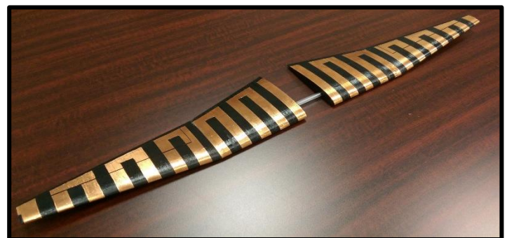
Figure 15. Foil antenna elements applied to 3D printed 15% scale G1X-B wing model
