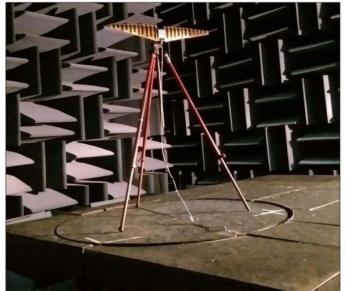
Figure 18. Antenna positioned in the anechoic chamber for testing.
