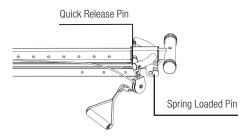
**B.** Take hold of the Vertical Column and pull it up until it is upright. Release the Spring Loaded Pin. You should hear it lock back into place. (**NOTE:** pin shown in picture is on right side.)
