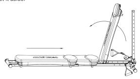
**3.** Next, pull the Spring Loaded Pin to release the Rail and fold the exerciser together as shown in Step 7 of TO STORE YOUR TOTAL GYM. Be sure you release the Spring Loaded Pin before folding.
