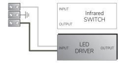
Controlled by bathroom lighting circuit
