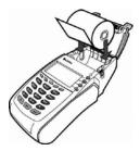
7. Close the paper roll cover by gently pressing directly on the cover until it clicks shut. Allow a small amount of paper to extend outside the cover (as shown below). CAUTION: To prevent damage to the print roller on the paper roll cover, always close the cover by gently pressing down on the paper roll cover.
