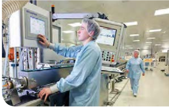
Specialist tubing for the medical technology industry is manufactured in the cleanrooms at Halberstadt, Germany
