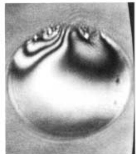
This view represents a fiber endface as viewed by an interferometer (50/125 micron coming fiber). The light/dark bands (fringes) indicate end face angle.
