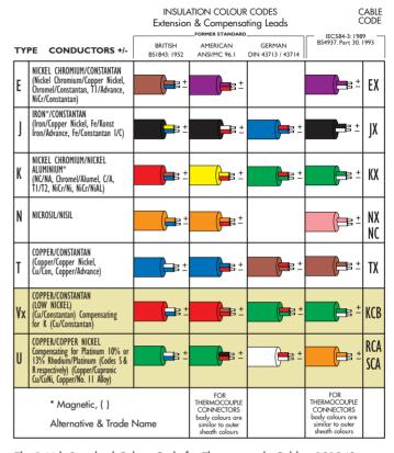
The British Standard Colour Code for Thermocouple Cables, BS1843: 1952 is superseded by BS4937 PART 30 1993 (=IEC 584-3 1989)
