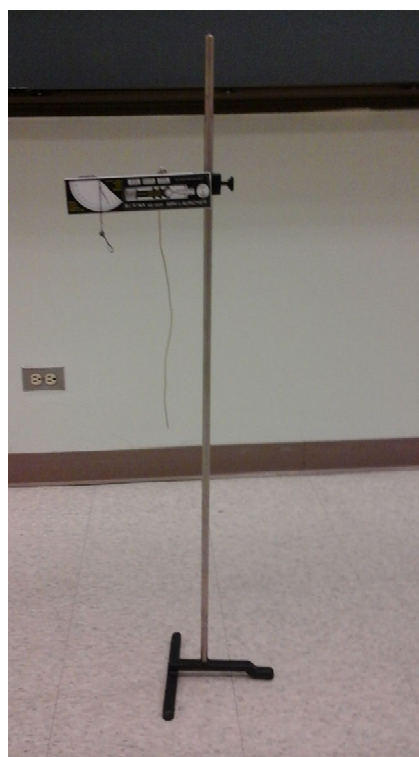
Illustration 1: When performing measurements such as range and launch height, always measure from the crosshatch, ie, the 'Ball Center of Mass' as shown in this picture.
