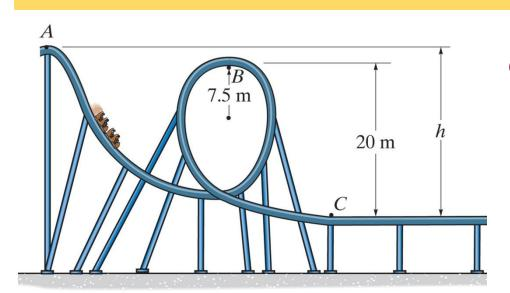
Given: The 800 kg roller coaster car is released from rest at A.
