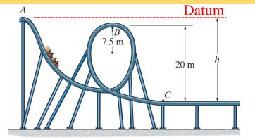
2) Find the required velocity of the coaster at B so it doesn't leave the track.
