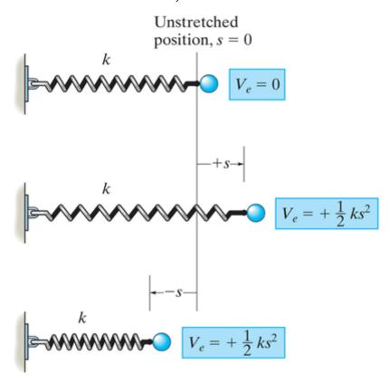
V<sub>e</sub> (where 'e' denotes an elastic spring) has the distance "s" raised to a power (the result of an integration) or
