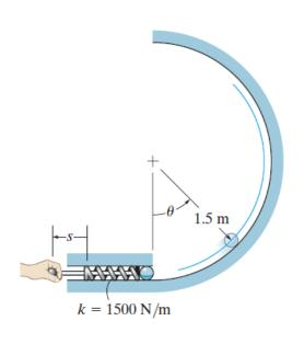
Given: The arm is pulled back such that s = 100 mm and released. When s = 0, the spring is
