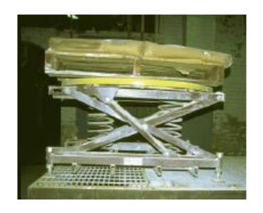
The weight of the sacks resting on this platform causes potential energy to be stored in the supporting springs.
