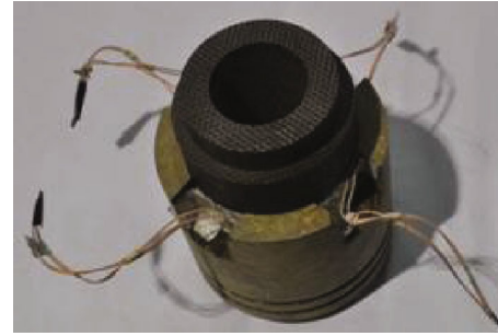
FIGURE 9: The throat insert bonded with strain gauges.
