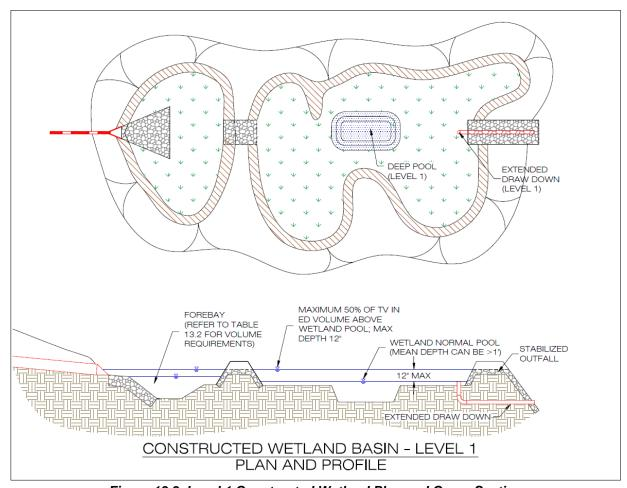
Figure 13.3. Level 1 Constructed Wetland Plan and Cross Section
