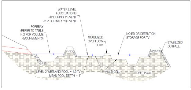
Figure 13.4. Level 2 Constructed Wetland Cross Section
