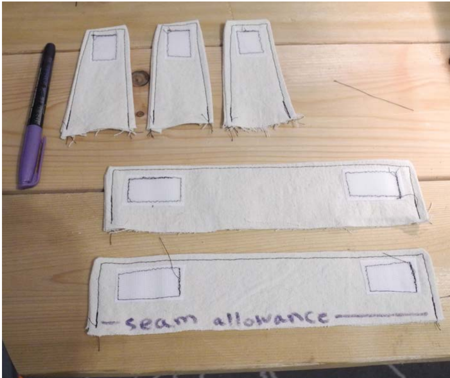
Illustration 11: Velcro size and location on tabs and flaps. Note: "Seam allowance" has been written on the flap as a reminder that the Velcro should be pushed near the folded edge rather than being placed in the centre.
