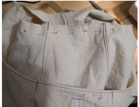
Illustration 26: Pinning the anorak hood to body. Note the short cotton "hangy loop" tails protruding past the seam.
