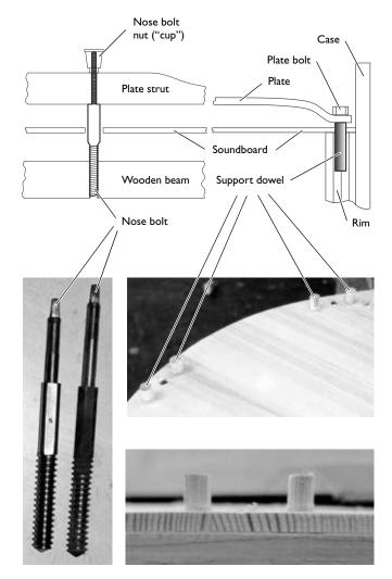
Figure 32 Piano plate supports: nose bolts and rim dowels.
