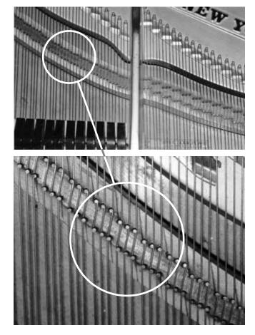
**Figure 109** This style of notching in a ca. 1900 New York Steinway concert grand model D creates unequal speaking lengths of strings in unisons in the mid-treble section. The purpose of unequal speaking lengths is to improve sustain in the "melody" octave.
