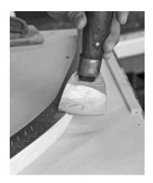
Figure 106 Cutting vertical separations between notches (Steinway & Sons factory, New York).
