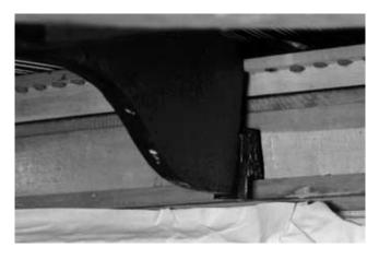
**Figure 36** The plate horn in modern Steinway & Sons grand plates is connected by a steel wedge to the metal shoe toe, which protrudes through the belly rail (see Figure 55 on page 29). The beams converge on the shoe behind the belly rail.
