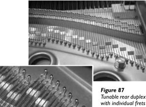
Figure 87 Tunable rear duplex with individual frets in each unison in a Fazioli 228 (courtesy Klavierhaus).
