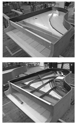
Figure 31 Installed grand soundboard with bridges (top) and plate (bottom) (Bösendorfer factory).
