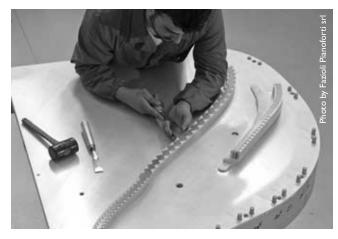
Figure 108 Bridges are notched sideways at the Fazioli factory.
