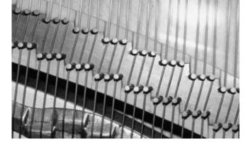
Figure 104 Notching of a replaced bridge cap.
