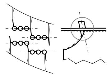
**Figure 105** Bridge notches on a new bridge (cap) should start somewhat closer to the center of the bridge instead of at the exact center of the bridge pins. This compensates for the grooves that form in the bridge cap over time.
