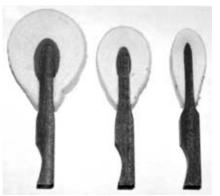
Figure 181 Hammers with unshaped and untapered tails.
