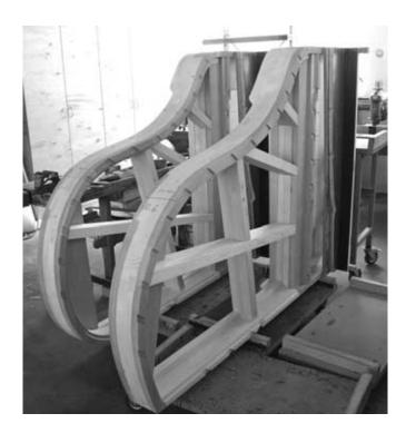
**Figure 30** Grand piano rims with beams and belly rails (Bösendorfer factory).
