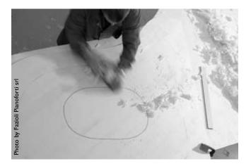
**Figure 119** Thinning the board toward the edges by hand (Fazioli factory).
