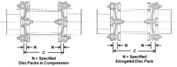
Disc Packs in Stressed Condition (Due to Compression or Elongation)
