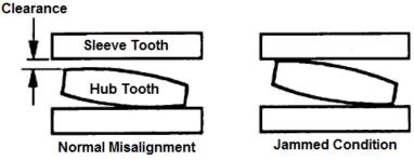
Gear Coupling Lock-Up Due to Excessive Angularity
