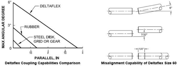
Capabilities of Deltaflex Coupling Compared to Conventional Coupling Designs
