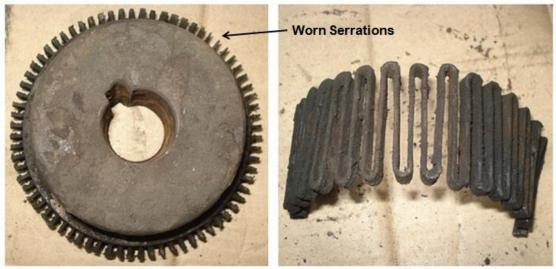
Hub Grid Wear of Grid Coupling Serrations Due to Loss of Lubrication
