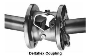
Deltaflex Coupling, patented design concept (U.S. Patent Number: 4033144) by Lovejoy is the real solution to installation, misalignment, and performance problems. The Deltaflex coupling can handle greater shaft misalignment without generating heavy reaction loads on the equipment shaft bearings. They are available in 5 basic sizes, from 10HP to 900HP.
