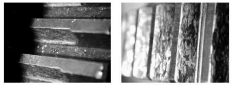
Sleeve Wear Wear on Hub Teeth Fretting on Sleeve and Hub of a Gear Coupling
