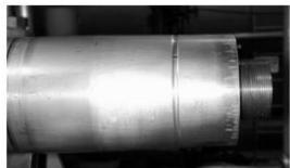
Keyless Hydraulically Dilated Coupling Shaft
