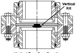
Vertical Type Gear Coupling
