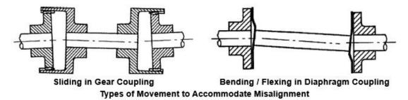
Above figure illustrates types of movement to accommodate misalignment - sliding in a gear coupling and bending or flexing in a diaphragm coupling.
