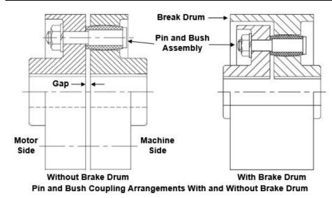
The coupling can be fitted with add-on parts such as brake disk or brake drum. Above figure shows typical coupling arrangements with and without brake drum. As shown in above figure, many coupling manufacturers provide guard on nuts for safety. Recommended amount of gap between coupling hubs is very important to compensate for shaft misalignment.
