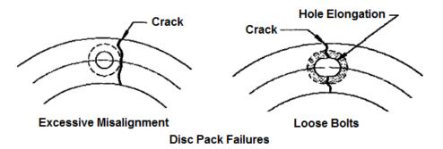
Above figure shows disc pack failure due to excessive misalignment and loose bolts. Due to excessive misalignment, cracks usually start on the outer discs and progress inward. If hole elongation and cracking is found, it is most likely due to loose bolting.
