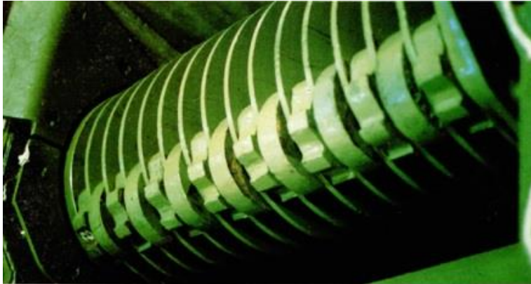
Each Row with Alternate Toothed and Plain Crushing Rings
