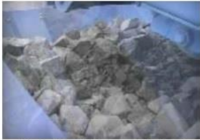
Choke Fed (Correct Method)
