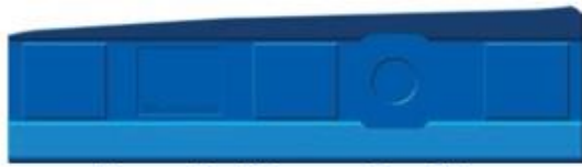
Excessive Wear on One Side
