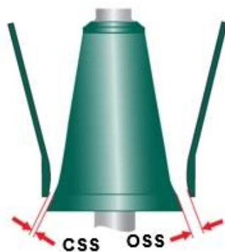
Open Side Setting of Gyratory Crusher
