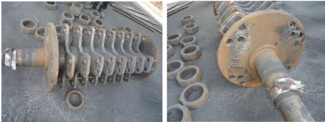
Damaged End Disc
