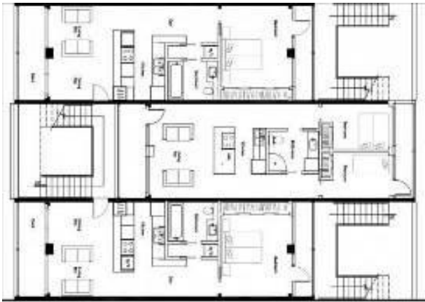
Fig 22: floor plan showing how it looks like if 3 containers are closed between each other.
