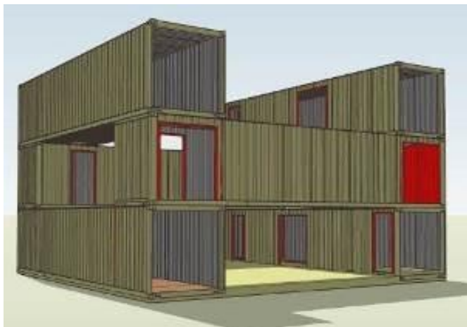
Fig 24: various configurations of staking the containers can lead to various models of residential units
