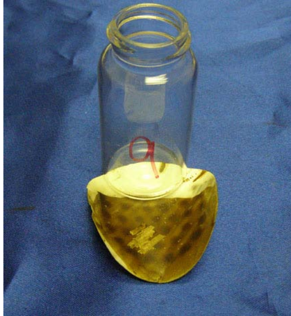
Figure 3-20. Photograph showing the collected solids for Sample 9, after solvent extraction and analysis.
