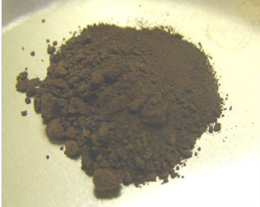
Figure 3-16. Photograph showing the collected solids for Sample 5, after solvent extraction and analysis.
