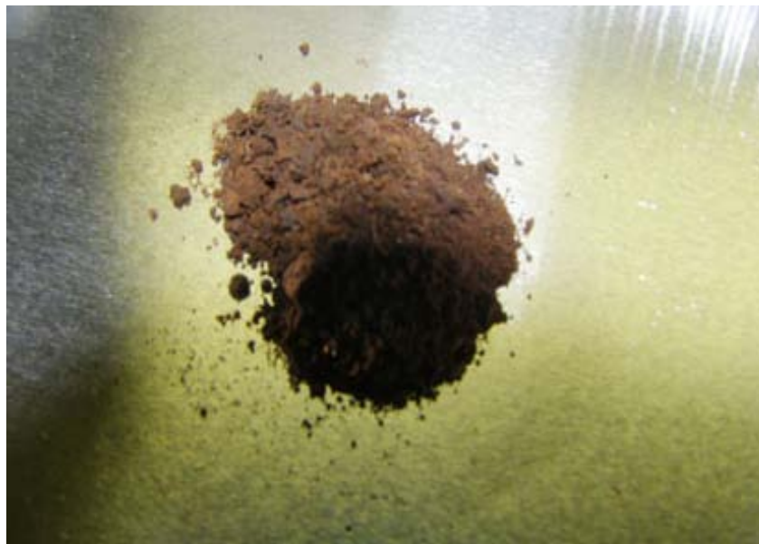
Figure 3-15. Photograph showing the collected solids for Sample 4, after solvent extraction and analysis.
