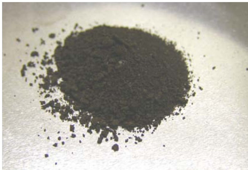
Figure 3-13. Photograph showing the collected solids for Sample 2, after solvent extraction and analysis.
