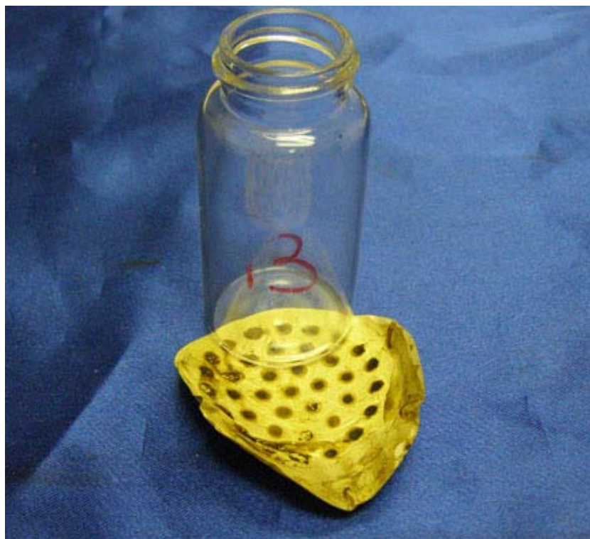
Figure 3-24. Photograph showing the collected solids for Sample 13, after solvent extraction and analysis.
