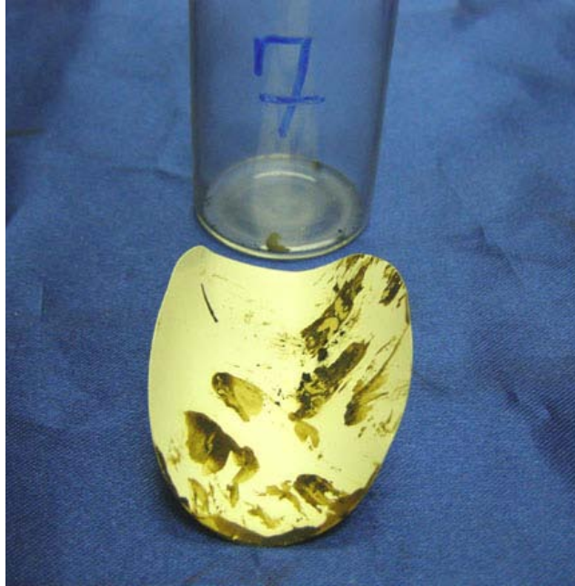
Figure 3-18. Photograph showing the collected solids for Sample 7, after solvent extraction and analysis.
