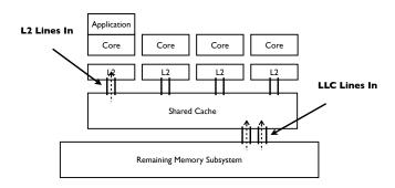
Figure 8: PMUs used for predicting contention characteristics
