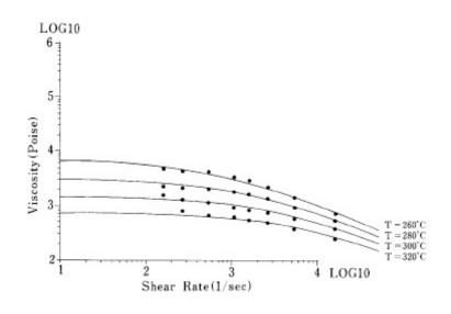
Fig. 5-2 Viscosity curve (Iupilon H - 3000)
