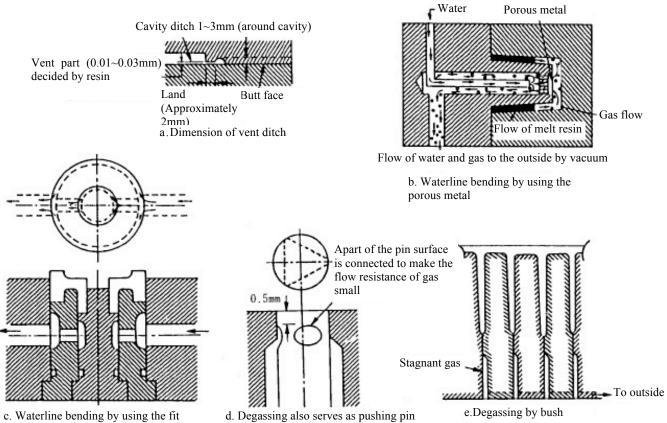
c. Waterline bending by using the fit clearance of the divided bush
