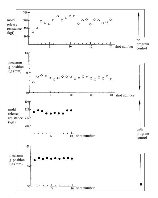
Fig. 1·3-4 Stabilization by the program control of plasticization process (Material: S-2000)
