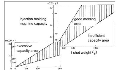
Fig. 1.1-2 Selection of molding machine from the injection capacity
