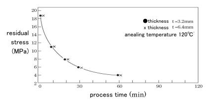
Fig.  $8 \cdot 1 - 1$  Annealing treatment time vs residual stress
