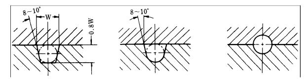
Fig.  $3 \cdot 2 - 2$  Cross sections of runners
