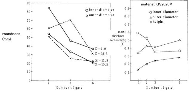
Fig. 4-5 Number of gate vs circularity (Relation to position of direction of height)
