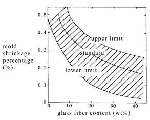
Fig. 4-1 Influence of glass fiber content to mold shrinkage percentage
