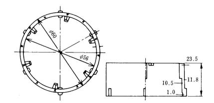
Fig. 4-4 Shape of molded piece and Position of dimension measurement
