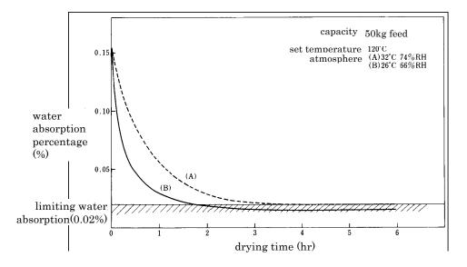
Fig. 2 · 1-2 Drying conditions by the hopper dryer
