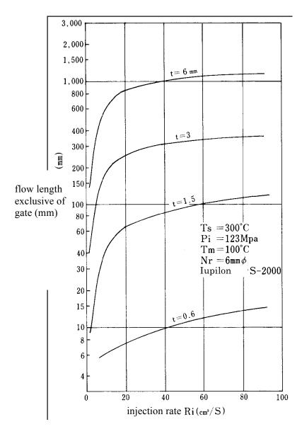
Fig. 2.2-1 Injection rate vs Flow length
