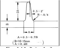
Fig. 3.1-8 Design of a rib
