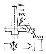
Fig.  $3 \cdot 2 - 9$  Example of submarine gate design
