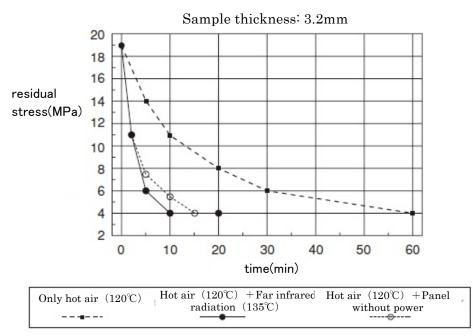
Fig.  $8 \cdot 2 - 1$  Residual stress decreasing curve of flat plate
