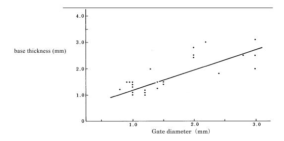
Fig.  $3 \cdot 2 - 7$  Actual relationship between the pin gate diameter and the thickness of the base The pressure loss at the gate of the circular section can be calculated by the following equation
