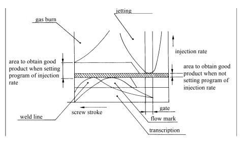
Fig. 1.3-2 Defective area of injection rate
