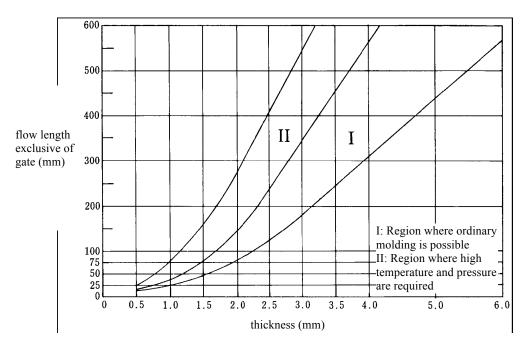
Fig. 3 · 1-1 The relationship between the wall thickness and the flow length for Iupilon / NOVAREX
