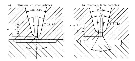
Fig.  $3 \cdot 2 - 6$  Shape and dimension of pinpoint gate
