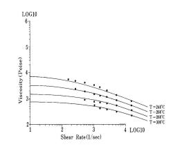
Fig. 5-1 Viscosity curve (Iupilon H - 4000)
