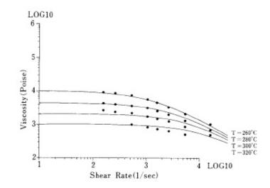
Fig. 5-3 Viscosity curve (Iupilon S3000)
