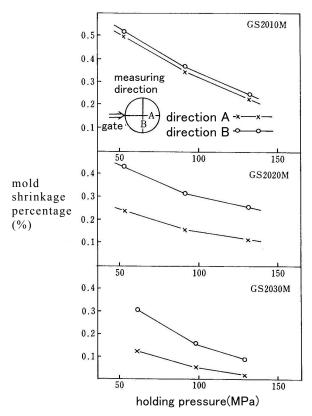
Fig. 4-2 Mold shrinkage percentage vs Holding pressure
