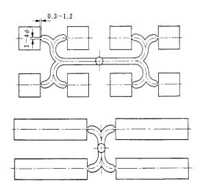
Fig. 3  $\cdot$  2 – 4 Parallel arrangement of cavities
