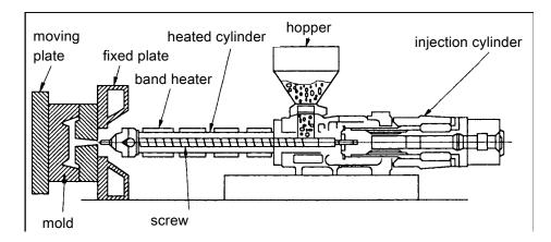
Figure  $1 \cdot 1 - 1$  Theory of the in-line screw type injection molding machine
