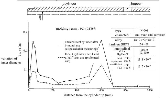
Fig. 1 · 1-3 Barrel material and abrasion data when using GF (30%) PC
