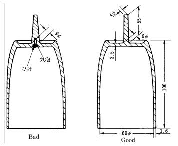
Fig.  $3 \cdot 2 - 8$  Examples of direct sprue design
