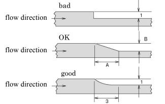
Fig. 3 · 1-3 Change of the thickness
