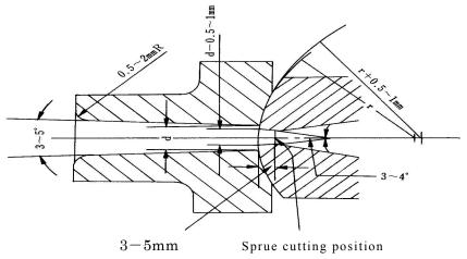
Fig.  $3 \cdot 2 - 1$  Shapes of the nozzle and the sprue bushing
