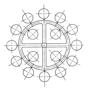
Fig. 3  $\cdot$  2 – 3 Circular arrangement of cavities
