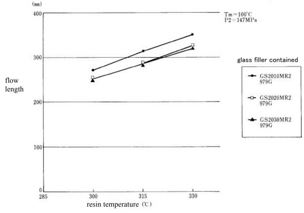
Fig. 3 • 2 – 11 Bar-flow flow length vs resin temperature
