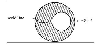
B. Reinforce the rib in the vicinity of the generated hole of the weld line.
