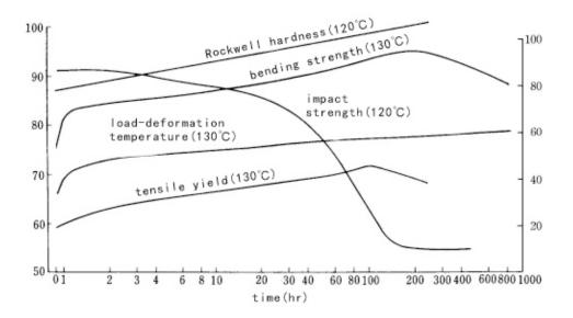
Fig.  $8 \cdot 1 - 2$  Change of physical properties by heat treatment of Iupilon / NOVAREX
