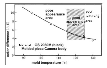
Fig. 1 · 4-1 Relation between the mold temperature and the appearance of glass fiber reinforced grade
