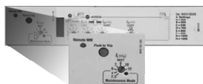
Close-Up of LG Trip Unit
