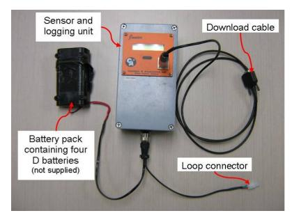
Figure 2: Bicycle recorder components
