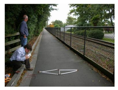
Figure 10: ZELT test loop and white box
