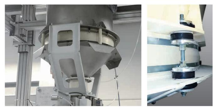
The BAV can be customized to accommodate different bulk material flow characteristics during discharging or refilling from bins or silos. In detail: the BAV Series 02 mounting dating from 1989.
