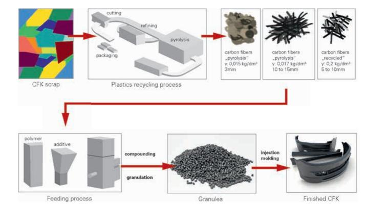
Recycling process of carbon fiber scrap with direct processing
