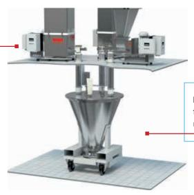
simultaneously feed three different additive products into a container in batches (LIW), generating a premix effect. The masterbatch is then moved to the batch mixer and added to the main product there (see figure).
