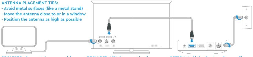
REQUIRED: Connect the coax cable to the TV "antenna/cable in" port.
