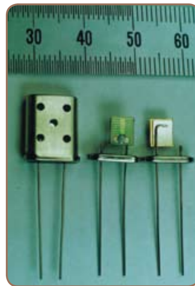
Capacitive humidity-sensitive element created by this technology
