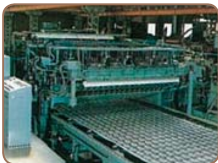
Plate 3D welding steel frame manufacturing system (fab deck panel)
