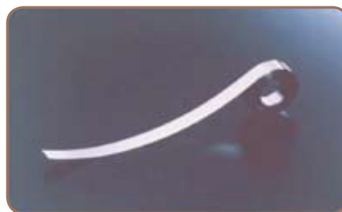
Fe-M-B nano crystal soft magnetic alloy thin band
