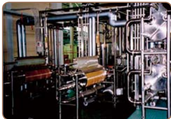
Membrane fractionation process system (UF apparatus)
