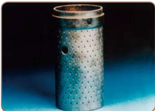
Example of ceramic-base composite material using silicon carbide fiber using this technology
