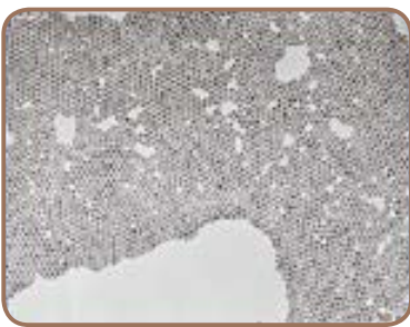
Image of independent metal super fines by transmission electron microscope
