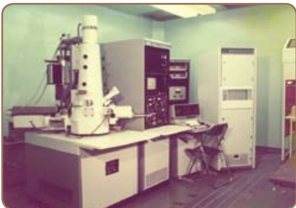
Electronic beam-exposure instrument draws a micro-electrode pattern up to 0.2 μm on a piezoelectric crystal wafer or dry glass plate. Also serves as an electron microscope.
