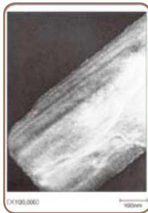
TEM photo of white conductive material
