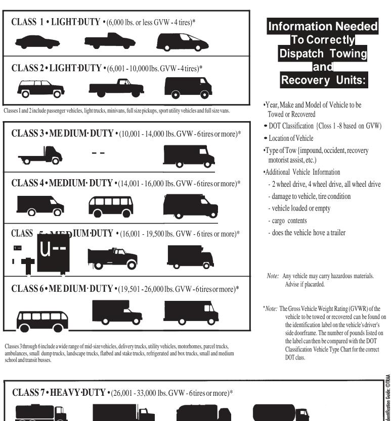
Classes 7 and 8 include a wide range of heavy vehicles, large delivery trucks, motor coaches, refuse trucks, cement mixers, all tractor trailer combinations including double trailers.
