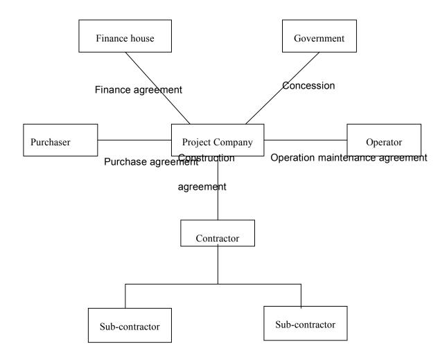
Fig.2-4 Build - Operate - Transfer
