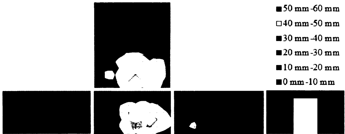
Figure 127 – Final Char Depths (mm) – Test 1
