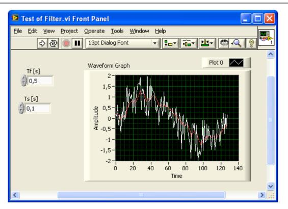
We see that the filter works fine. The red line is the unfiltered sine signal with white noise, while the red line is the filtered results.
