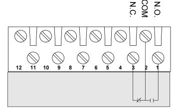
Figure 3. Connections for shorted SCR detection relay.
