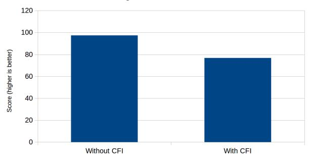
Figure 5.1: CoreMark results with and without CFI. Default settings, 1000 iterations
