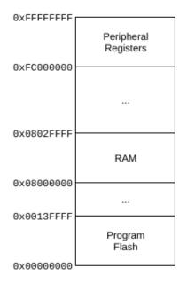
Figure 2.1: Simplified memory map for RM46L852 processor [1]
