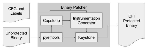
Figure 3.2: Overview of binary patching system
