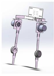
Fig. 1 Exoskeleton structure of lower limb
