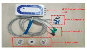
Fig. 2 EMG acquisition equipment
