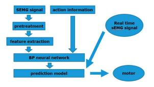
Fig. 8 Control process
