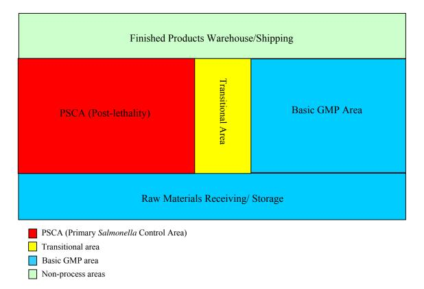
Figure 2-3. Example of a conceptual plant layout showing three process areas with different hygiene control: a Primary *Salmonella* Control Area (PSCA) in red, a transitional area in yellow, and a basic GMP area in blue. The non-process area (e.g., warehouse, shipping) is in green (offices and employee welfare areas are not shown). This layout may be applicable to products such infant formula.
