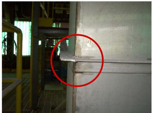
Figure 3-2. A flat surface that can collect product (This should be eliminated or sloped).
