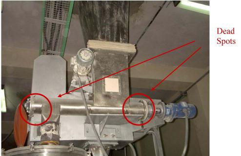
Figure 3-1. Ends of a horizontal screw conveyor – always a potential area of stagnant product build-up.
