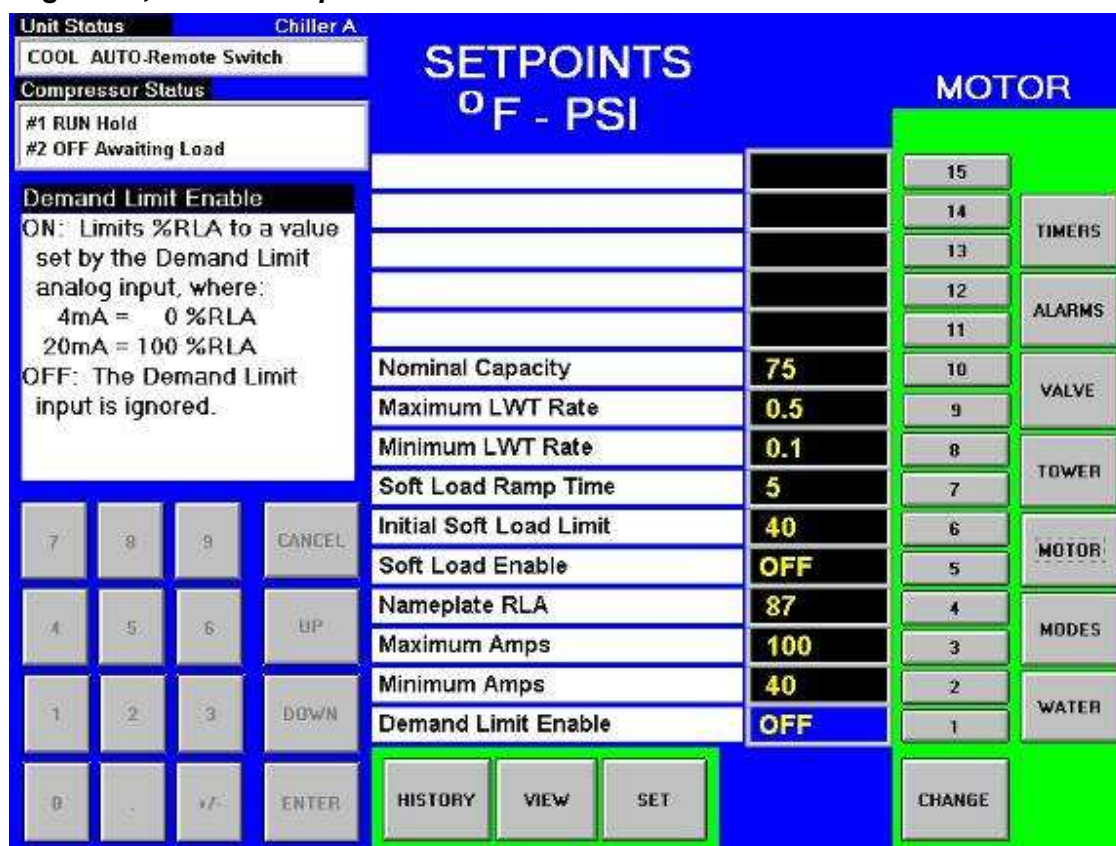
Figure 23, MOTOR Setpoint Screen
