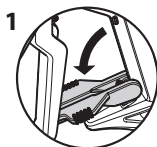
Gun locked (gun will not spray)
