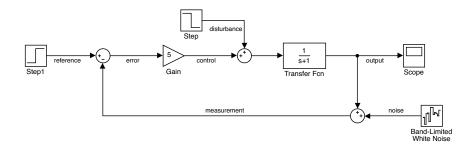
• The control input tries to move the system in a direction that is opposite to the error, and is proportional to the error in magnitude.
