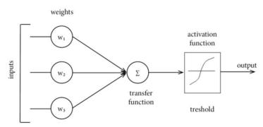
Fig.6 Basic elements of an artificial neuron. [16]
