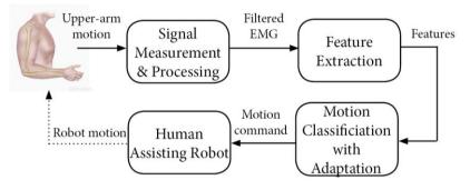
Fig. 11 EMG-based upper arm robot control system
