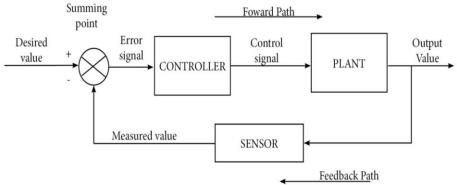
Fig. 1. The closed loop system
