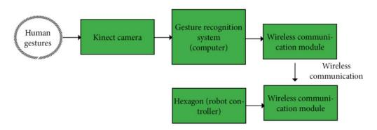
Fig.9. The system structure of the robot control system based on gesture recognition. [19]
