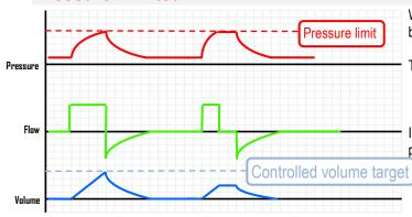
When pressure is limited, the pressure limit will be maintained if it is reached before the end of inspiration.
