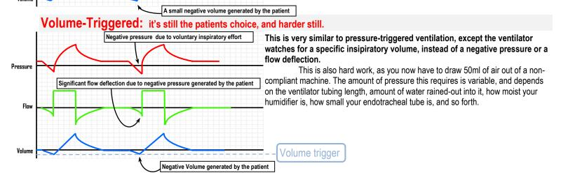
The machine has a set respiratory cycle time, and a set I:E ratio (ratio of inspiration to expiration).
