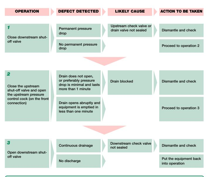
N.B. : In normal operation the appliance must not present any permanent pressure drop. Otherwise dismantle and verify.
