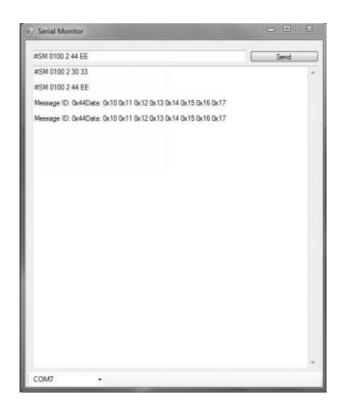
In this case, we sent two CAN Messages with the same ID (0100) but different data. Next, we received to messages through my standard test configuration (i.e. USB-to-CAN gateway with Windows monitoring tool as the second CAN node).
