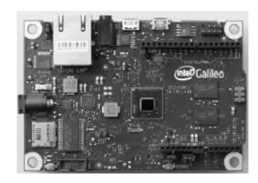
The Intel Galileo is a microcontroller board based on the Intel<sup>®</sup> Quark SoC X1000 Application Processor, a 32-bit Intel Pentium-class system on a chip. It is designed to be hardware and software pin-compatible with Arduino shields designed for the Uno R3.
