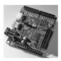
As similar as it may be to the Arduino, the differences are what really make the Maple stand out. It harnesses the power of a 32-bit ARM Cortex-M3 clocked at 72 MHz to push 39 GPIOs, 16 analog pins, 12-bit ADC resolution and 15 PWM pins at 16-bit resolution. In order to make sure you have plenty of programming room to flex that hardware, the Maple also provides 128k Flash and 20KB SRAM. All of this performance is delivered in the same form factor as the Arduino Pro.
