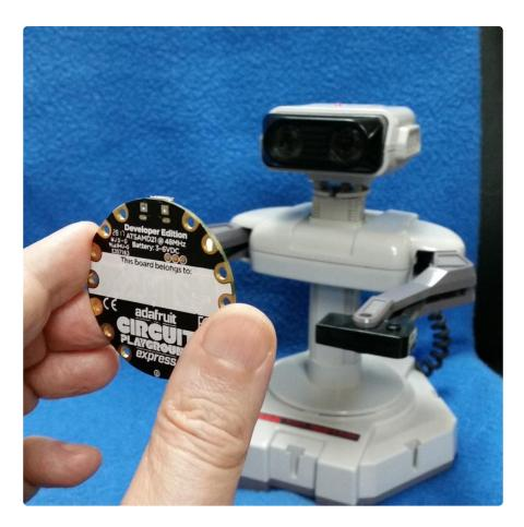
If you have issues with R.O.B. not responding to the LED commands, carefully open the head up and remove the paper which restricts light to the left eye and blocks the right eye. This will allow more LED light in and make him easier to control.
