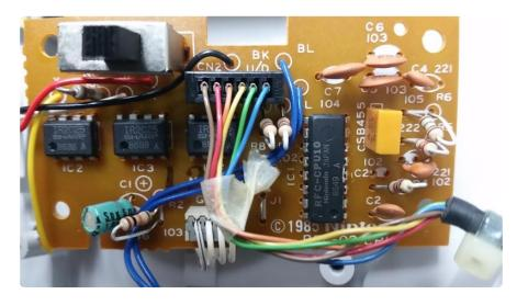
The Sharp IR2C25 chips are undocumented motor control drivers. The RFC-CPU10 is a custom Nintendo microcontroller or programmable chip that is also undocumented. The 6 wire rainbow wiring harness goes to the midsection via a coiled cable. The 4 wire white harness leads to the head section. The slide switch disconnects the battery power from the rest of the circuitry when in the off position.
