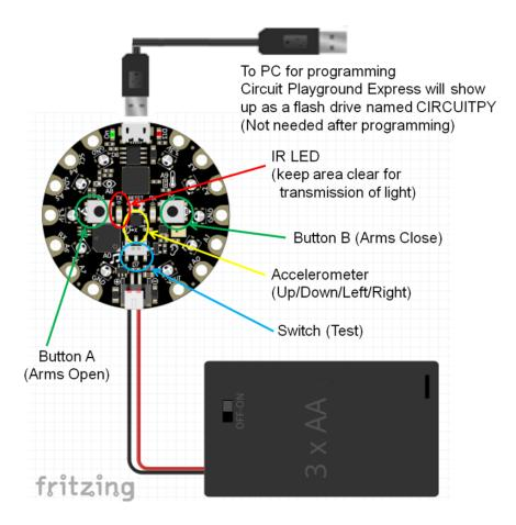
For programming and testing, you don't need the battery pack connected, the USB cable will power the Circuit Playground Express and allow for programming.
