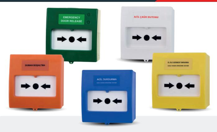
Designed to be connected to any brand of conventional fire detection systems. Internal 470-ohm resistance allow ease of installation. It is suitable for flush and surface mounting. An optional transparent protective cover can be installed. It is easily resettable via special key.
