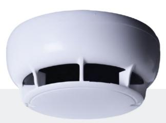
TFD-3240 Conventional heat detector uses two NTC for precise measurement of the environment to detect fire. Detector classified as A2S and will report an alarm at 55°C.
