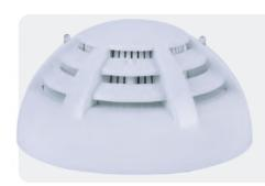
TSD-701 is a natural gas detector which can be connected to conventional fire alarm systems (NO) and Intruder alarm systems (NC) or to be used as a stand-alone device with 12-24V external power supply.
