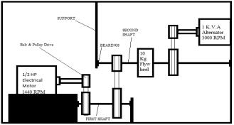
Fig. 3: Schematic Layout of our System
