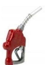
The OPW 118® Series is designed for use in retail and commercial filling applications including prepay, self and full service, credit/debit card readers or card-lock systems to help prevent gasoline spills. The OPW 118® will not open until the pumping system is pressurized, and closes automatically when the pressure is removed.
