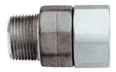
Designed for use with fuel oil nozzles (at inlet only), the OPW 36S provides 360° swivel action. The full-circle swivel reduces the physical strain of aligning the nozzle with the fill pipe. Available in ¾" and 1".
