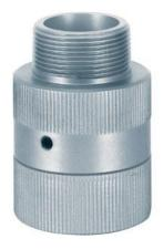
Designed for use with fuel oil nozzles (at inlet only), the OPW 25 provides 360° swivel action. The full-circle swivel reduces the physical strain of aligning the nozzle with the fill pipe. Available in 1  $\frac{1}{4}$ " and 1  $\frac{1}{2}$ ".
