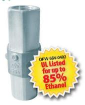
The OPW 66V Series breakaways are designed and rigorously tested for use in today's fuels. Installed on fuel dispensing hoses, they will separate at the designed pull force, reducing expensive damage to the dispenser and piping system. Internal dual valves close automatically during separation stopping the flow of fuel from both the dispenser and the separated hose, reducing environmental and health risks of potential spilled fuel. Available in ¾" and 1".
