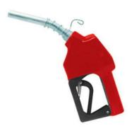
The OPW 11AF® Nozzle is a sturdy industry proven standard used primarily for fueling up to 15 gallons per minute. The 11AF® is an automatic dispensing nozzle designed for use in transfer pump. This nozzle should not be used for retail applications, and does not include a No Pressure – No Flow Device.
