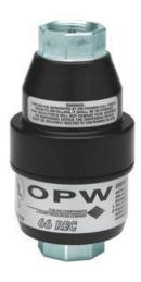
The OPW 66REC is the first dry reconnectable breakaway for the conventional dispensing market. It is designed to be installed on fuel dispensing hoses, and will separate when subjected to a designated pull force. The dual valves seat automatically, stopping the flow of fuel and limiting any fuel spillage, while protecting the dispensing equipment. When reconnecting the separated halves, the 66REC seals tightly on an O-ring before the poppet stems engage to open the valve.
