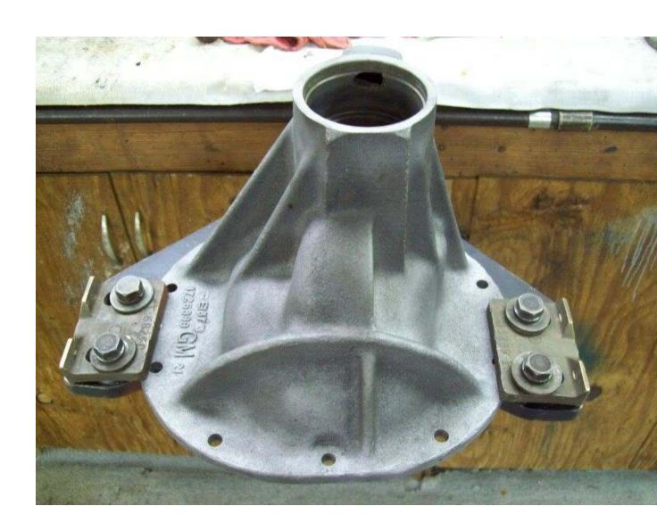
Once the case is cleaned and blasted, it is much easier to read the casting numbers and casting date on the driver side of the case and the ratio code and assembly date (AB 523-May 23) on the passenger side.
