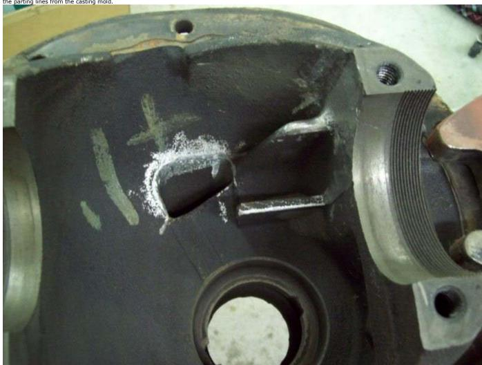
The next step is blasting the case inside and out. I concentrate blasting on the areas where the grinding was done just to make an even finish all over. This step is not necessary, but this is how I do it.
