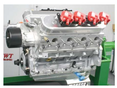
While the conventional mounting location for the coilpacks is over the valve covers, keep in mind that this isn't written in stone. If you want to clean up the valve cover areas, simply relocate the coilpacks elsewhere under the hood, using longer plug wires and extending the harness wires.
