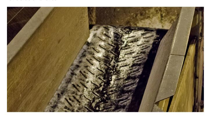
For your inclining conveyors, we offer a wide range of **profiled belts**. Our profiled belts are often used for wood chips and parcelled goods in inclining conveyors. Our **U- and V-shaped cleated belts** are well suited for conveying e.g. gravel and crushed stone, and for inclining conveyors where cover profiling is not sufficient. Depending on the application, a large range of profiles and types of rubber are available.
