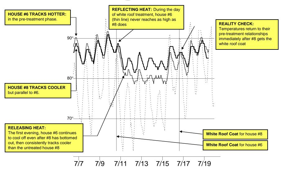
Tracking the effects of white roof coating on two identical homes
