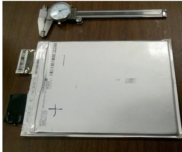
Figure 2-1 Lithium-ion Phosphate Battery Cell
