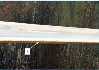
Figure 14: Fan Blade- The fan blades were found with a considerable amount of wear and pitting in the fiberglass. Detail point one refers to pitting on the leading edge of the fan blade that is caused by water droplets invading the plenum.
