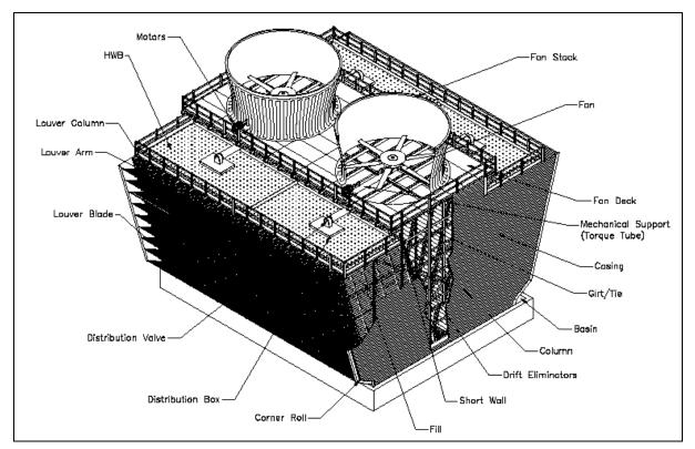
Figure 5: Example cross-flow cooling tower schematic
