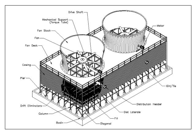
Figure 6: Example counter-flow cooling tower schematic
