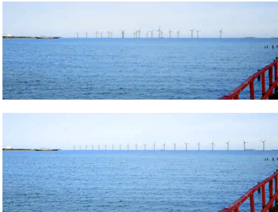
Figure 4 The Middelgrunden “27 turbines in three rows” and “20 turbines in a curved line” seen from the beach at Kastrup [11] and [12]
